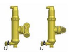
If space around the pipe on which the Turnable needs to be installed is limited, the clip that holds the separator and the rotating base together may be removed, allowing the front part to be detached. Once the threaded base is installed on the pipe, the front part can be re-attached and fixed again by re-inserting the clip from the top.
