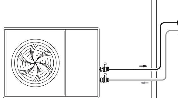
**Diagram 1:** Example of direct install onto a heat pump unit. The valves can also connect directly onto the anti-freezer valves or HP hoses.
