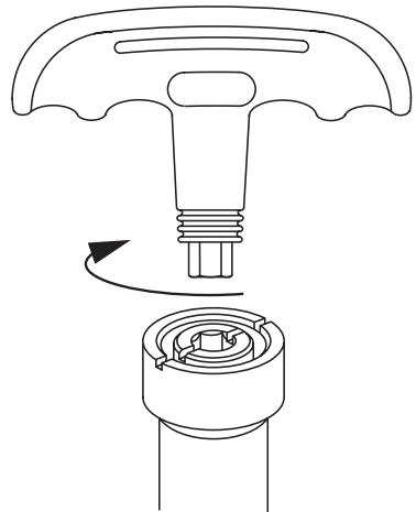
**Diagram 2:** The ball valve features a quarter turn adjustment spindle that can be adjusted using the allen key tool provided.
